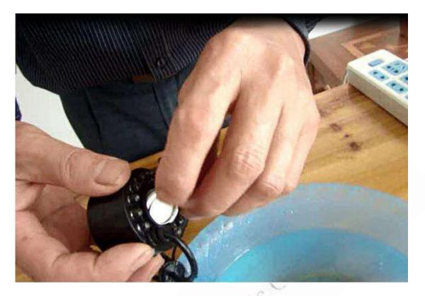
3) change the new piezoceramics. turn the black part clockwise to tighten the bit as picture.
