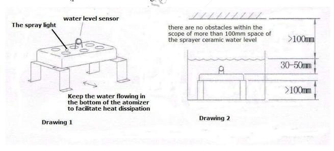
2. The Spray indicator light will be bright after connecting the mist maker with power supply, then the ultrasonic atomizer will work.
