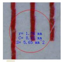
4) Circle-diameter: click <sup>☉</sup>, left-clicking to choose a start point for a circle; draw the circle to an end point, release the mouse, and the radius of the circle will be displayed.
